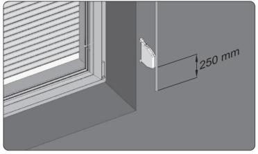
3. Lower the blind shutter armor, then cut the tape to a length of 250 mm below the assembly site of the retractor.
