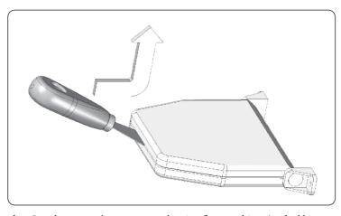
1. In order to open the tape retractor housing, flat screwdriver (preferably a spatula) should be inserted into the gaps in the front part of the casing, and evenly
