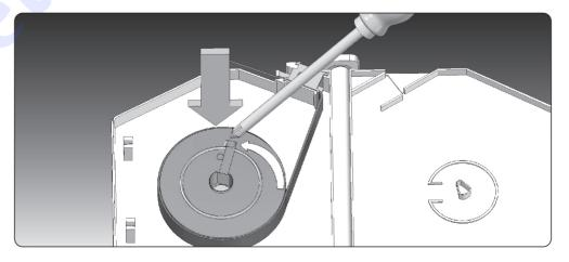
7. Undo the reels. Use a screwdriver to press the locks and allow the strap to be wind back automatically
