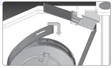
6. End the tape to the hook that protrudes from the reel spool.
